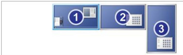
In this example, I have a dual display adapter and an external USB Display adapter I purchased from DisplayLink. It will hook up to any USB and with the correct drivers drive an extra monitor. On this machine I monitor a log file that needs monitored all the time so I swiveled the monitor sideways.
